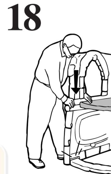
**Ilus. 17 - 20** To attach threshold to the walls, position each end of threshold under each wall. Push down on walls until threshold pops in place.
